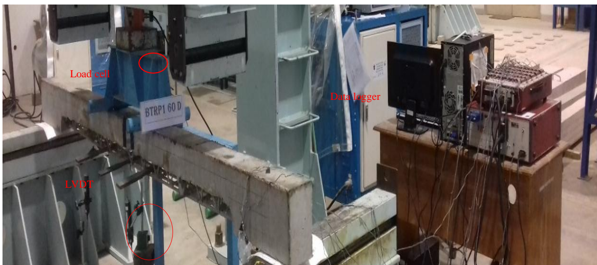
Figure 6. The photograph of setup tests.
